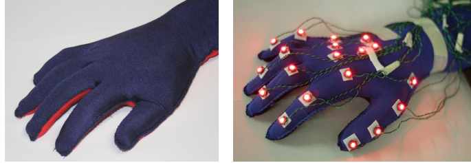
Fig. 3 The sensing glove used in our study (on the left) and the sensing glove with added markers (on the right).
