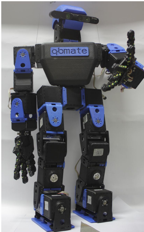
Fig. 11: Torso and legs of humanoid robot using VSA.
