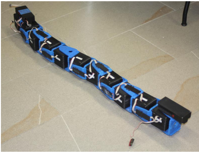
Fig. 10: Snake robot conformed by VSA.
