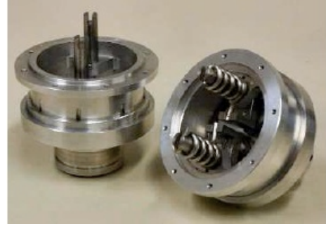
Fig. 3. An open view of the VSA-II prototype (from [10]); there is one such device for each motor on the two sides of the driven joint
